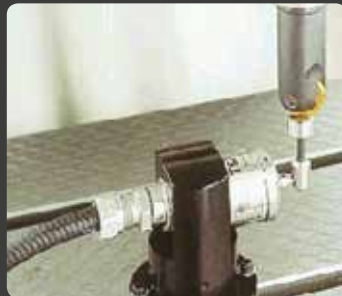
Tool probing with touch probe
